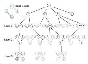
Figure 2: A portion of a vertex-induced subgraph tree with 3 levels. Lightly colored subgraphs are removed from consideration by automorphism checks.
