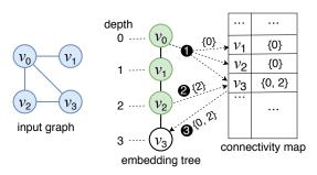
Figure 6: An example of connectivity memoization. **0**, **2** and **3** are timestamps to show the order of actions.
